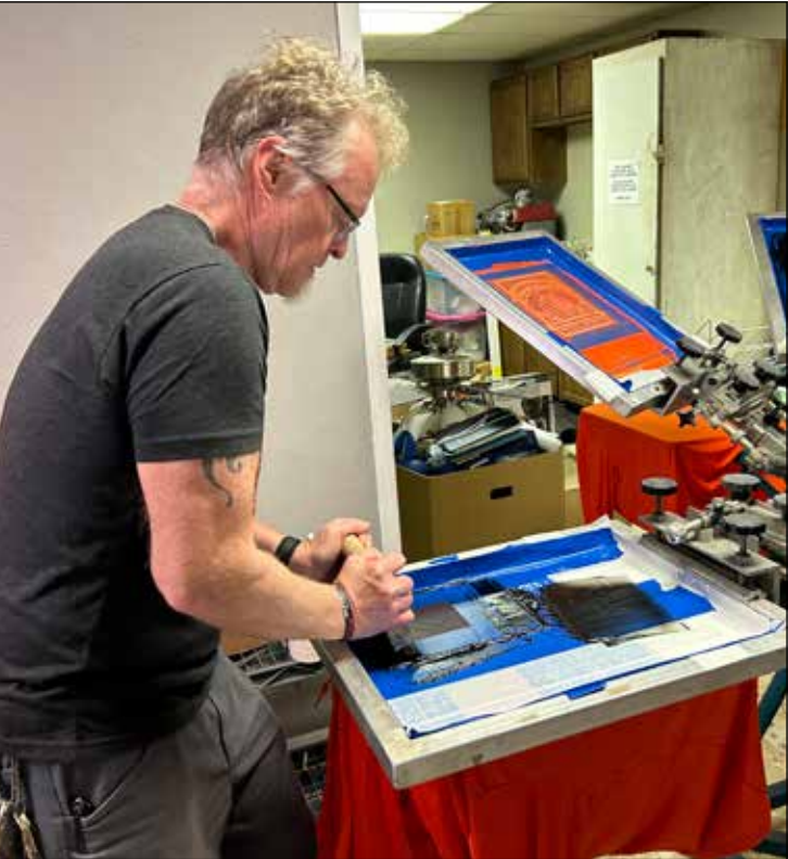
Screening the black color on an orange shirt before it goes through the dryer. If it needs a different color it goes to the next unit to add that layer.
