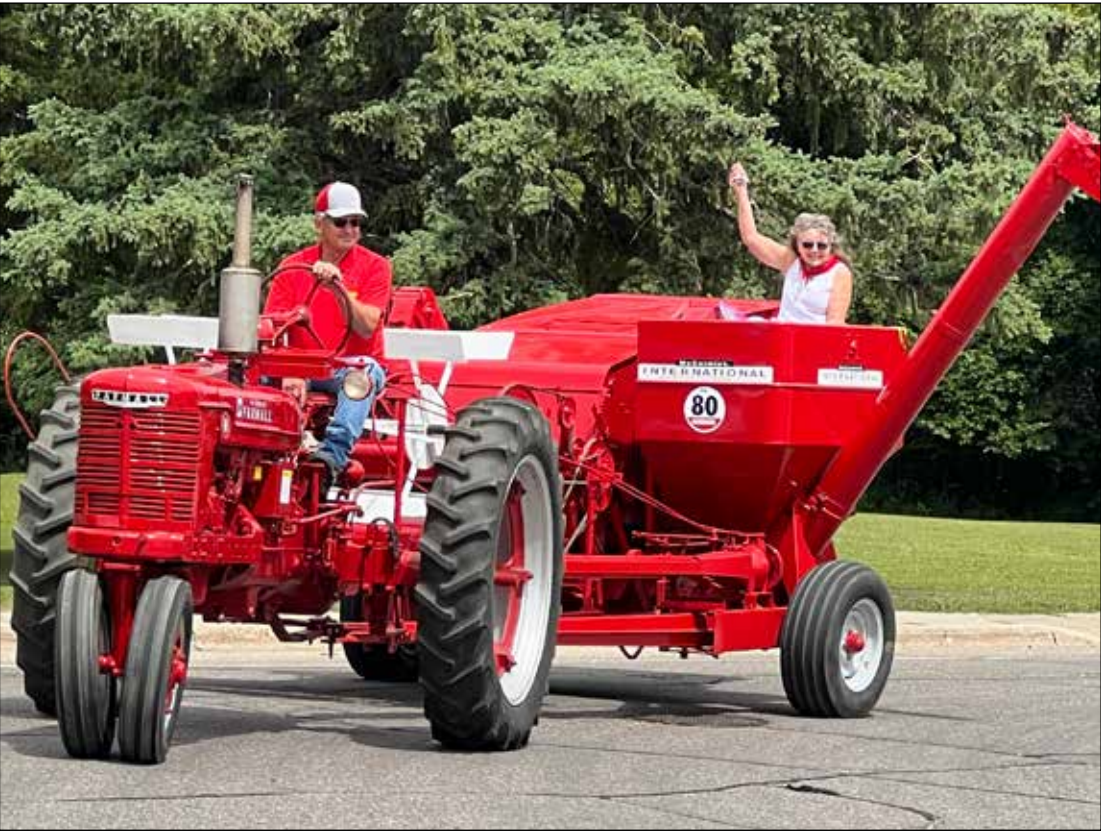
This is an International H tractor towing a #80 International pull-type combine with a 6 ft. straight head. Vernon Johnson, from Clearbrook, bought the tractor from Albert and Victor Erickson, from Clearbrook. The combine was purchased from Eugene Lange, from Gonvick. Then Vernon began restoring both the tractor and the combine. Vernon passed the two pieces of equipment to his brother, Robert Johnson of Clearbrook. Robert is driving it today in remembrance of Vernon who passed away on a cold December day in 2019. Marilyn Johnson was busy throwing out beans, corn and candy at the Gonvick Lions Rodeo parade.
