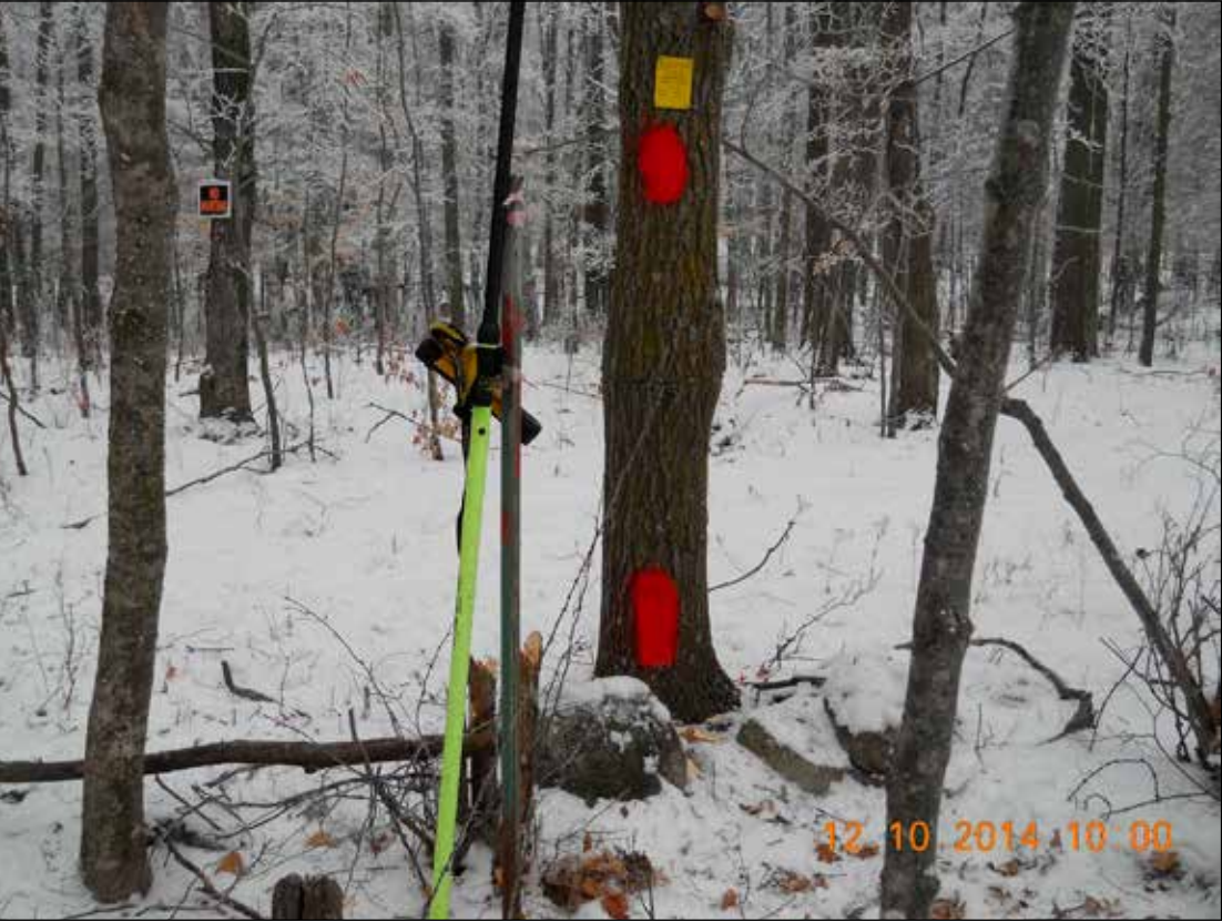
Bearing trees are marked in this way: double blaze painted orange, plus corner location tag.
