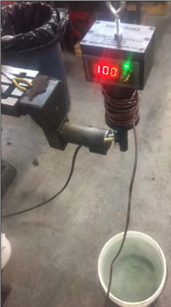
After working out the mechanic's of the best teaser on the market, Terry Strom came up with the Smart Teaser which had an adjustable rpm and a LED display.
