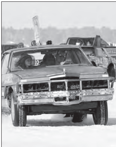
#5456 #86 Chad Tabaka's ice racer clearly shows the "Studded" front tires for traction on the ice and passengers are allowed in the ice racers.
