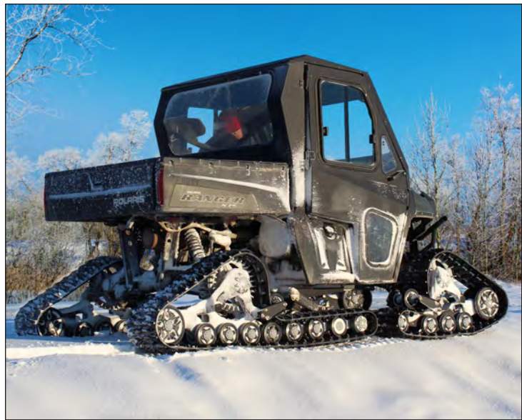
The Maxim track, designed for UTVs, nearly doubles the track area with its unique switch back system.
